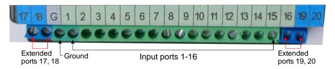
The *Ground* must be connected to the ground of the module that provides the input signals. Usually this will be a current detection module such as the Okkie or OkkieNext.
