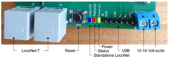
The USB interface (CH340) must be connected to an USB port on the PC. This also allows the LocoNext to be supplied with power. This interface must be ordered separately!
