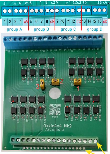
16 outputs to LocoNext All screwterminals or 18 Dupont pins The LocoNext and the OkkieNext4x4 make a perfect combination for occupancy feedback. The coupler board (available with and without LED bar) connects both modules without any problems.
