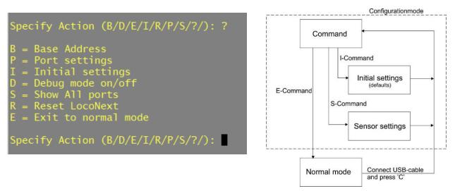
Each command consists of a single letter and does not need to be terminated with <enter>. The letters are based on the English description of the function of each command.
