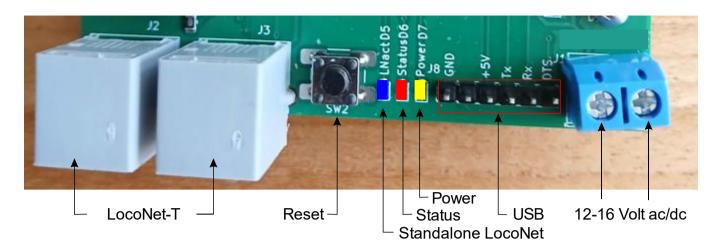
In configuration mode, the status LED is always on. In Normal mode, it is off and flashes briefly when sending LocoNet signals. In stop mode, it is also on.
