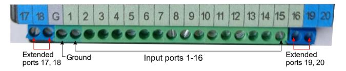
The *Ground* must be connected to the ground of the module that provides the input signals. Usually this will be a current detection module such as the Okkie or OkkieNext. This can also be done via a ground loop.
