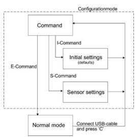
Each command consists of a single letter and does not need to be terminated with <enter>. The letters are based on the English description of the function of each command.
