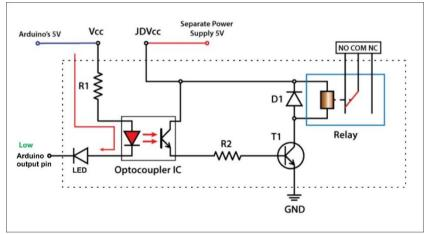
In this picture you also see that the relay is energized when the Arduino port is LOW.
