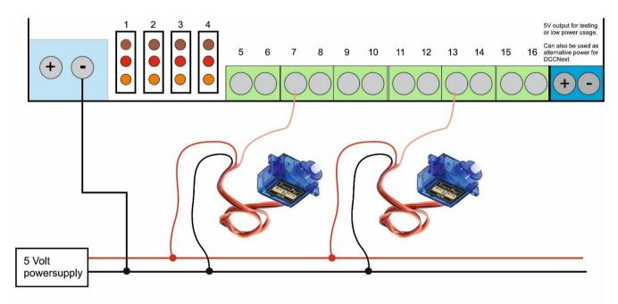
Connecting servo's with screw terminal and 5V ring lead
