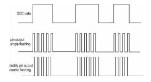
In **mode 3**, the port is alternately high and low as long as the DCC data is high. The on and off times are separately adjustable between 5 and 30,000 ms. (=30 sec.)
