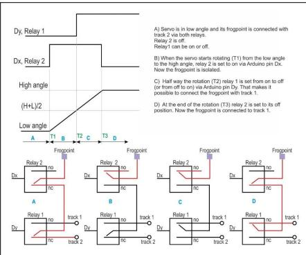
the switch. You can also use the relay to switch something different then the frog point. Actually, the frog port is simply a port that becomes high or low at the same time as the switch is switched.
