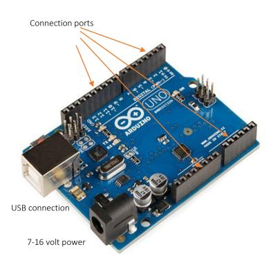
An Arduino port has an output voltage 0 or 5 volts and can process a maximum of 40 mA. For accessories that require more power (such as motors, alternating coils and LED strips) an additional amplification stage is required.
