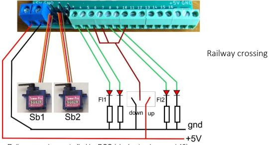
Railway crossing controlled by DCC (single steady on port 10) or manual with toggle switch.
