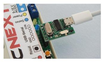
This decoder can be equipped with both screw terminals and Dupont ports. A servo can be connected directly to the ports. A separate 5V servo power supply is also provided for this.
