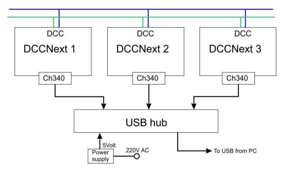
With this USB option, you do not need to mount the power supply circuit.
