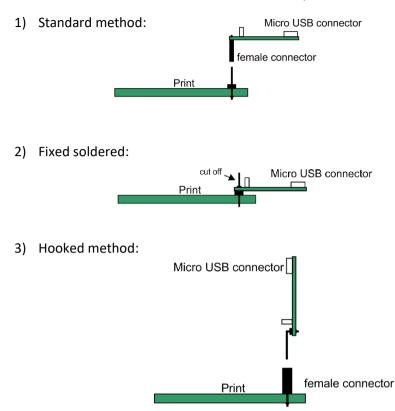
This method saves space. The danger is that the interface is set up incorrectly; so with the USB connector on the other side.
