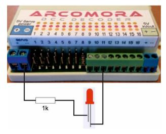
7. Connect a led with in series a resistor of about 1k between the gnd of the servo power and a port.
