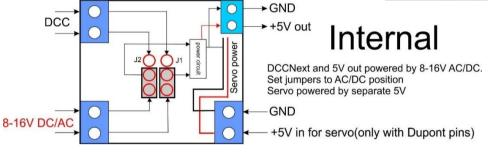
2) **DCC**. The DCCNext is powered by the DCC signal connected to the DCC terminal. The LocoNet Railsync signal can NOT be used.
