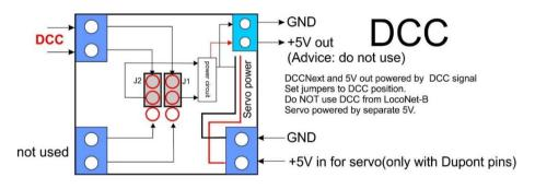
3) **External**. The DCCNext is powered from the blue 5 Volt terminals. This can be a low power supply.
